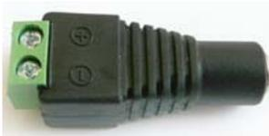
The wires can be connected to the output of the power supply with the the DC Adaptor supplied (5A is the maximum load that should be put on it), alternatively you could use a terminal block, or bullet connectors. Whatever the connection method it should be located in the dry. The Module/s will only light if connected the right way around with the + output of the power supply to the + input of the Modules, these are usually printed on the Module.
